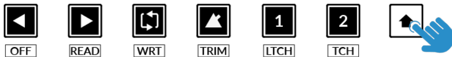
STEP 2: Engage the SHIFT KEY to re-purpose the secondary transport keys to be automation keys.
