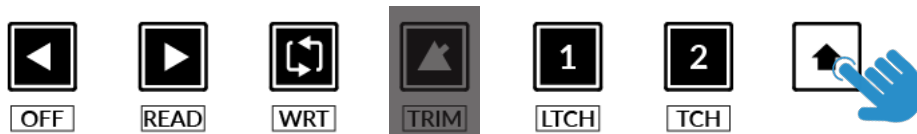
STEP 2: Engage the SHIFT KEY to re-purpose the secondary transport keys to be automation keys.
