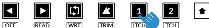
STEP 3: press to select the automation mode you wish to set the track to.
