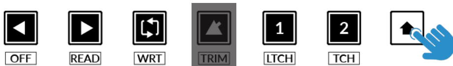
STEP 2: Engage the SHIFT KEY to re-purpose the secondary transport keys to be automation keys.
