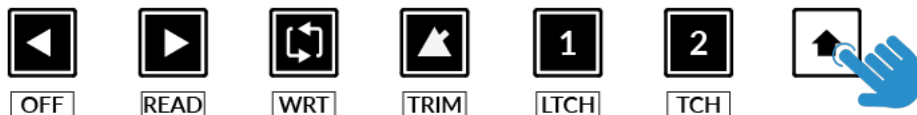
STEP 2: Engage the SHIFT KEY to re-purpose the secondary transport keys to be automation keys.
