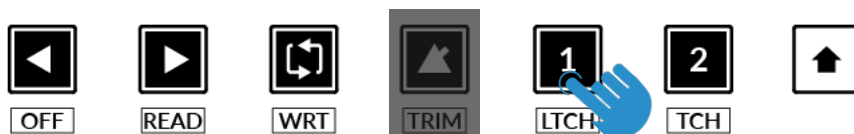
STEP 3: press to select the automation mode you wish to set the track to.
