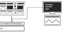
TCA can be deployed as a backup control surface for mission-critical applications, without the physical requirements of a traditional console. Utilising System T's Dormant Backup feature, TCA can take control of active audio processing in an instant, through a single button push.
