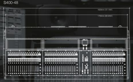
S400 is a fixed layout control surface that is available in 16+1, 32+1 and 48+1 fader configurations.
