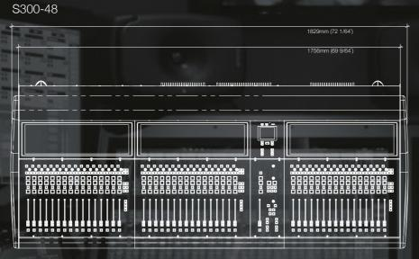
S300 is a fixed layout control surface that is available in 16+1, 32+1 and 48+1 fader configurations.
