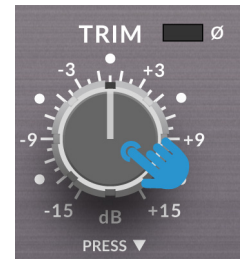
Channel 1 TRIM Relay disabled
