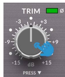
Channel 4 TRIM Auto Standby enabled
