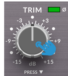
Channel 1 TRIM Relay enabled
