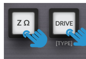
Channel 4 Buttons ZΩ decreases timeout, DRIVE increases timeout
