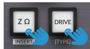
Channel 2 Buttons +ZΩ decreases brightness, DRIVE increases brightness
