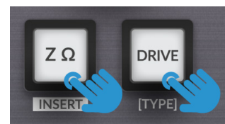
Channel 1 Buttons +ZΩ decreases brightness, DRIVE increases brightness
