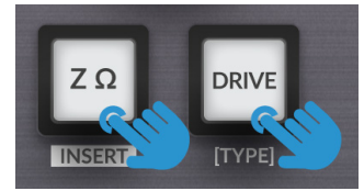
Channel 1 Buttons +ZΩ decreases brightness, DRIVE increases brightness
