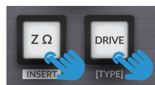
Channel 8 Buttons ZΩ decreases timeout, DRIVE increases timeout
