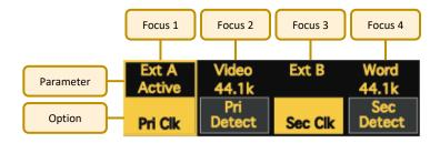
The lower half of each focus box displays the option to be changed, the upper half displays the parameter it is currently set to. Turning the **SELECT** encoder moves the focus window across the 4 sections.
