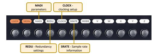
The Options menus are accessed by individual buttons to instantly navigate to the desired settings page on the OLED Display. The front panel must be unlocked for these buttons to function.
