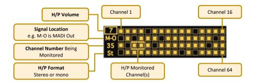
By default when entering the monitoring page the encoder will adjust the headphone volume. Pressing the **SELECT** encoder will move the focus to alter **Signal Location**. The options are:
