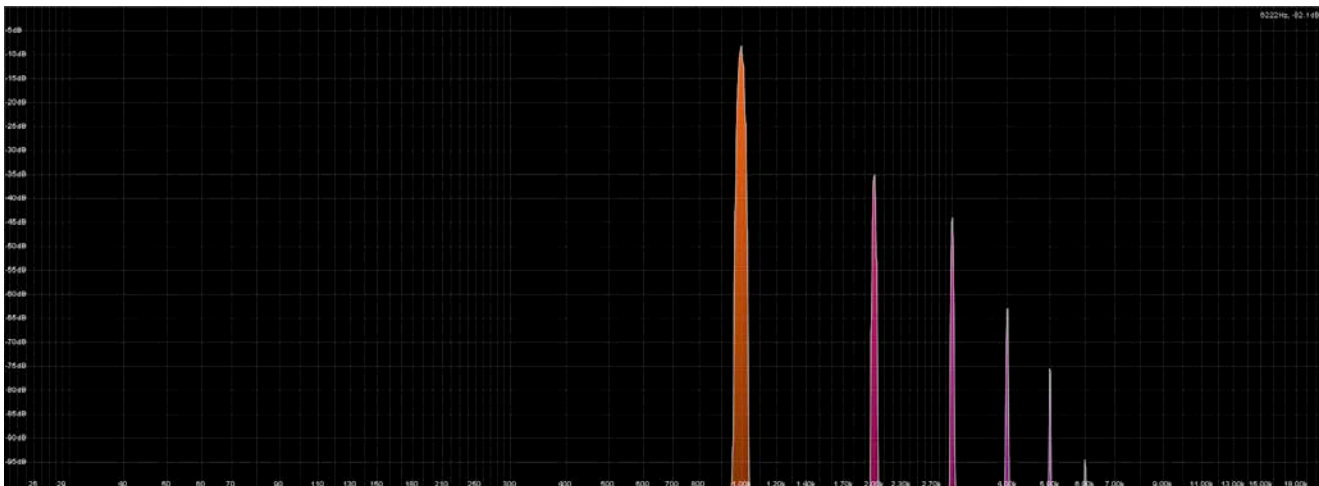
Example of additional harmonics generated using a 1kHz tone. ('Low' Density)
