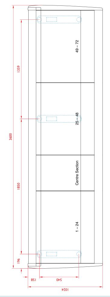
**96 CHANNEL FOOTPRINT** (Centre section can be positioned to the right of any channel bay)
