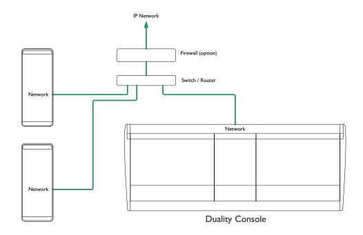
To ensure minimum latency, the ipMIDI driver uses multicast UDP rather than TCP/IP. This means that the network connection should be as short as possible and should only use routers that can support high data transfer rates. Problems have been experienced with some domestic routers, particularly when used with Pro Tools.
