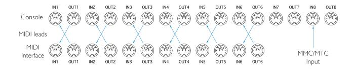
MIDI ports should be connected to your DAW MIDI interface unit – three available ports are required (one port includes an IN and OUT socket). To connect a port, the output of the MIDI interface unit port I should connect to the MIDI I input port on the console and the MIDI output of the console port I should connect to the input of your MIDI interface unit port I. Repeat for the other ports using the diagram above as a guide.
